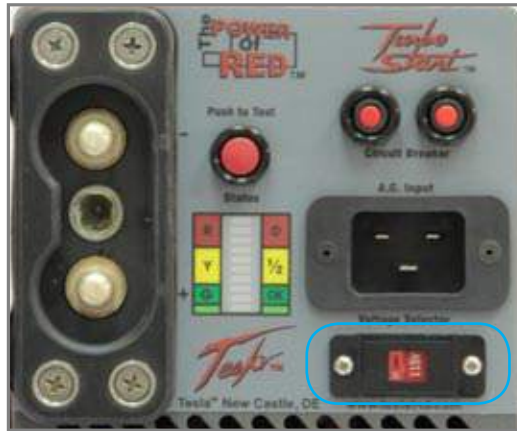
Figure 2.10.1 Input Voltage Selector Switch (outlined in blue)
