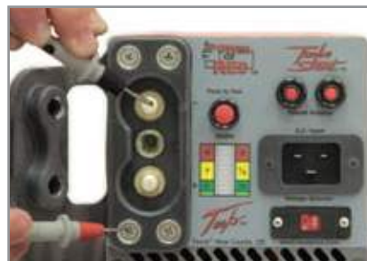
2. Place the positive probe to the fastener screw on the dc Receptacle. Move the negative probe to the dc negative post. Multimeter should read 0 Volts.
