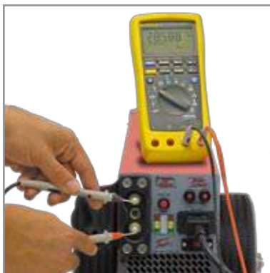
Figure 3.8.2 – Testing DC Receptacle
