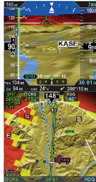
Pro PFD — Evolution Synthetic Vision top, terrain view with hazard overlay bottom
