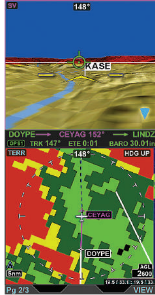
MFD Split Screen Layout — Evolution Synthetic Vision top, navigation and top-down terrain hazards bottom
