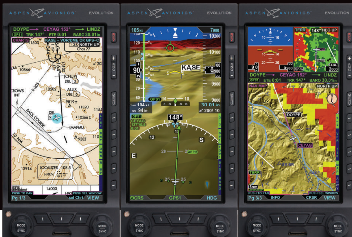
Evolution 2500 showing Evolution Synthetic Vision on center PFD
