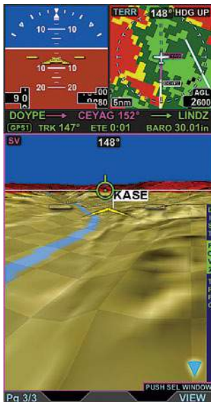
MFD Thumbnail Layout — secondary AI and top-down terrain hazards at top; Evolution Synthetic Vision bottom
