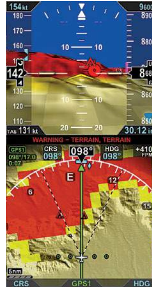
Pro PFD — Evolution Synthetic Vision with terrain warning top, terrain view with hazard overlay bottom
