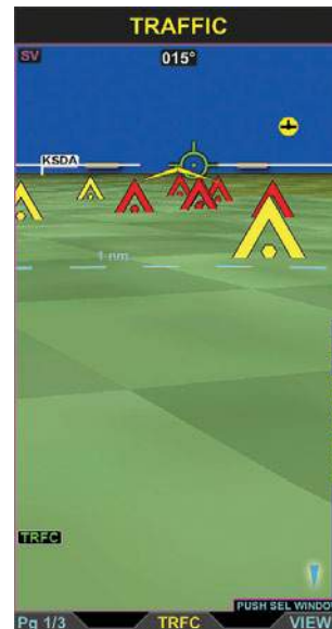
MFD Full Screen Layout — Evolution Synthetic Vision, narrow field of view, 3D traffic
