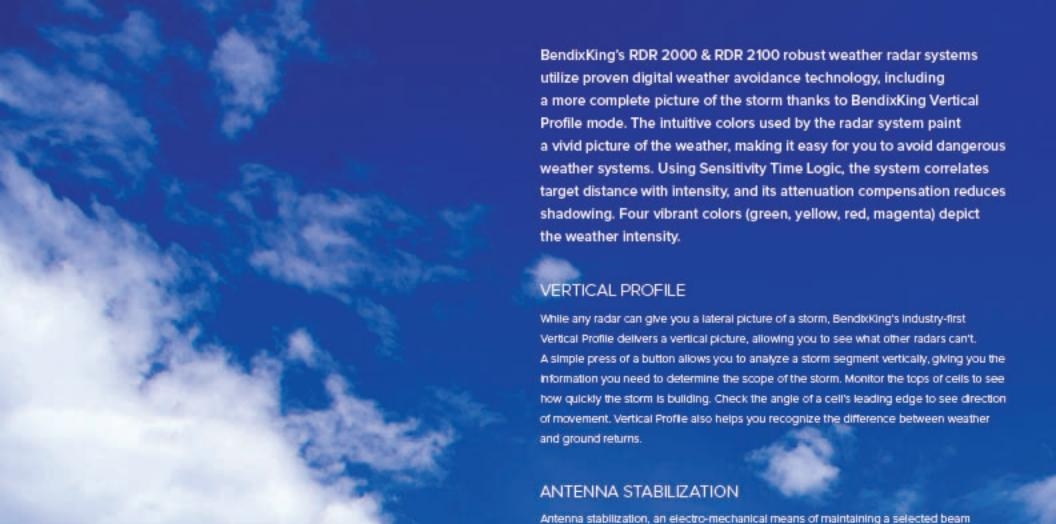
relative to the earth's horizon, keeps your screen clear of ground returns during moderate aircraft maneuvers. Select from two antennas, 10-inch or 12-inch, to fit a wide variety of airframe applications. The RDR 2000 & RDR 2100 systems accept ARINC 429 digital
