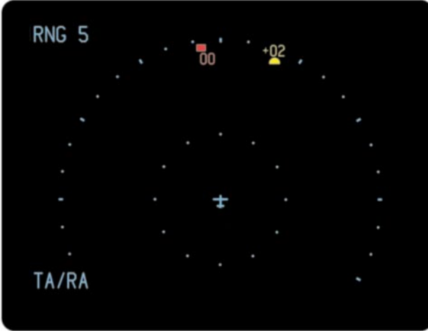
TA and RA traffic off scale, 5 mile range, TCAS Only Mode.
