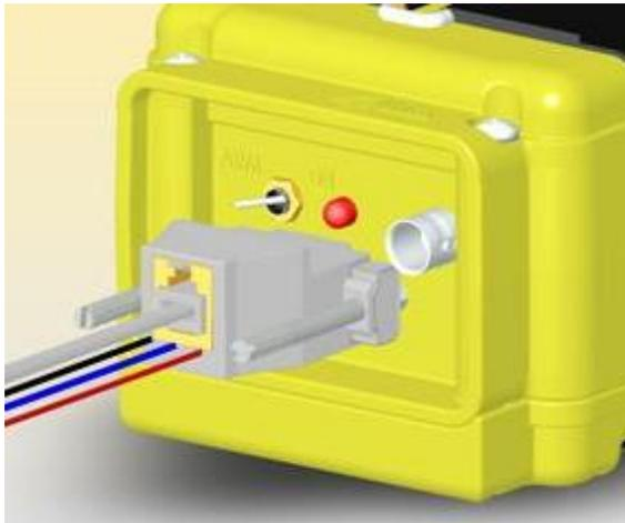
**Figure 10: Module Interface to ELT Connection**
