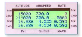
Held Remote Control, the Touch Screen Remote Control or a wireless Bluetooth connected PDA. All the important air data functions are simultaneously displayed on all interfaces, constant screen or menu changes are not required. Readings of both commanded and measured test values are displayed.
