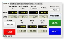
Laboratory testing can also be performed by a PC connected via RS232 to the remote hand terminal connector. The comprehensive manuals include all the control instructions. ADWIN software is available as a ready-to-run PC based interface.
