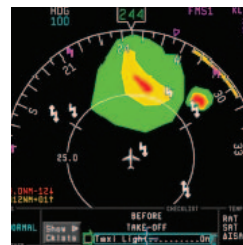
Lightning detection system
