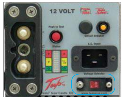
Figure 1.3.4 – TI1530 GPU-12 Input Voltage Selector Switch
