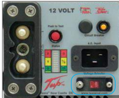
Figure 2.10.1 Input Voltage Selector Switch (outlined in blue)
