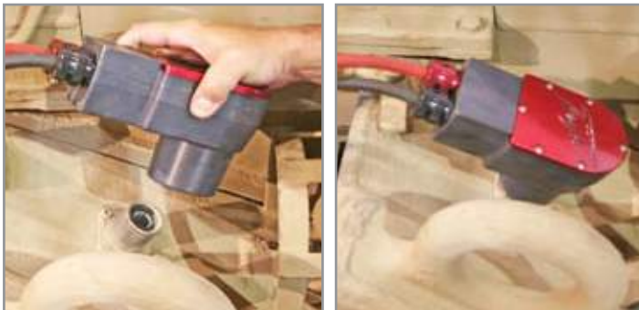
Figure 3.11.2 Attaching NATO DC Power Cable to vehicle
