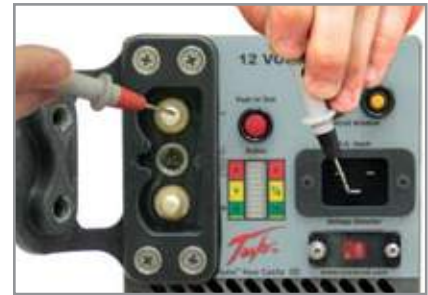
3. Move the positive probe to the DC negative post. Multimeter should read greater than 10 MΩ.
