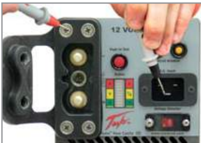
4. Move the positive probe to the fastener screw on the DC Receptacle. Multimeter should read less than 1Ω.
