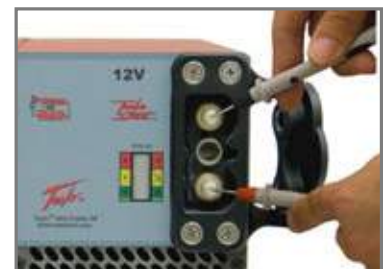
3.8.8 - Measuring Voltage on DC Output Connector
