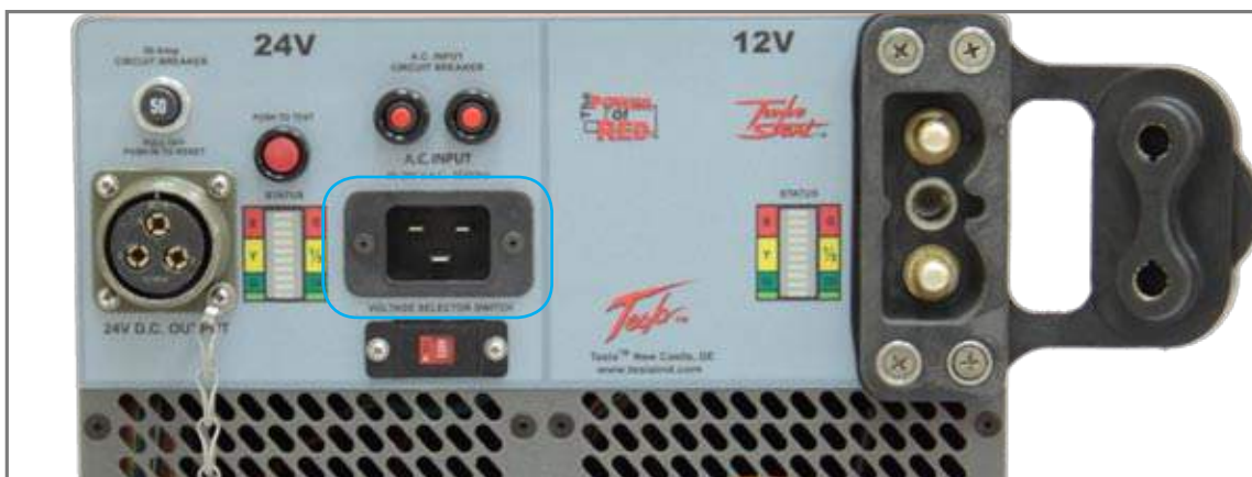
Figure 2.9.1 - AC Input Connector (outlined in blue)
