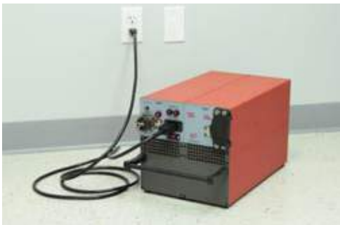
Figure 4.3.1 Connecting TI1550 12-24-UAV GPU to AC Power Supply
