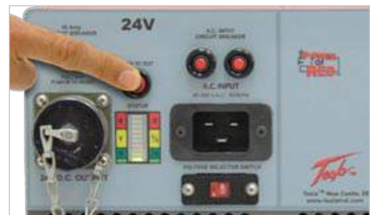
"Push to Test" Status Meter Indicators
