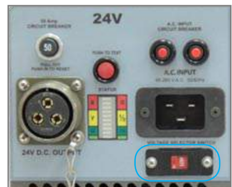
Figure 1.3.4 – TI1550 12-24-UAV GPU Input Voltage Selector Switch
