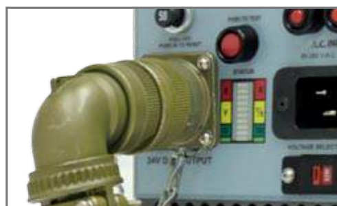
Figure 2.10.1 - 24 Vdc Output Connector (outlined in blue) /12 Vdc Output Connector (Outlined in red)
