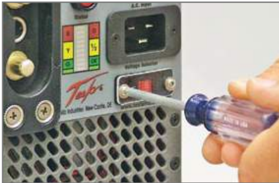
Figure 2.13.2 - Unscrew Protective Cover
