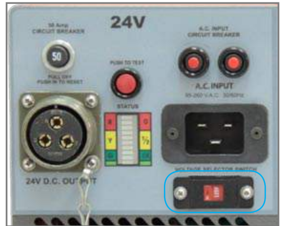
Figure 2.13.1 Input Voltage Selector Switch (outlined in blue)
