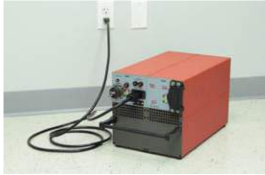
Figure 3.12.1 - Connecting TI1550 12-24-UAV GPU to AC Power Supply
