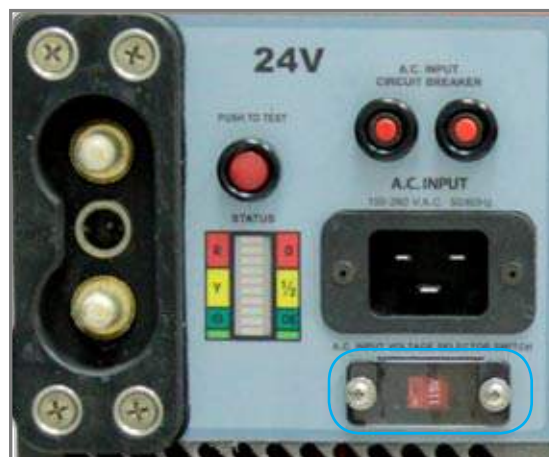
Figure 2.12.1 Input Voltage Selector Switch (outlined in blue)
