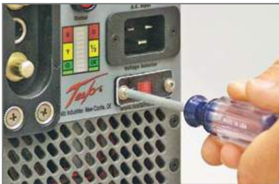
Figure 2.12.2 - Unscrew Protective Cover
