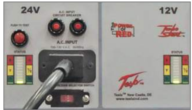
Figure 3.12.2 - AC Power Connected with LEDs Illuminated
