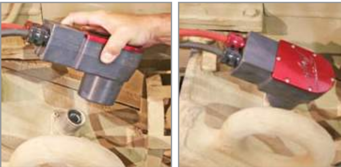
Figure 3.11.2 Attaching NATO DC Power Cable to vehicle
