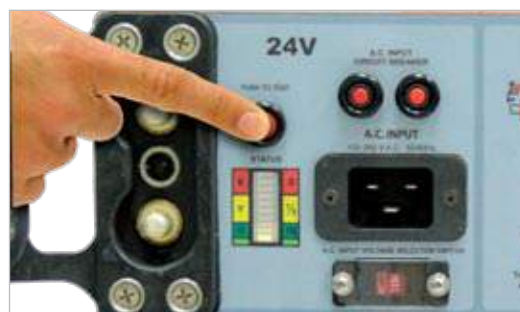
"Push to Test" Status Meter Indicators
