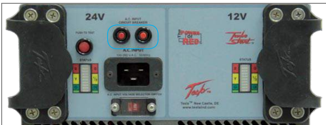
Figure 2.8.1 - AC Input Circuit Breaker (outlined in blue)
