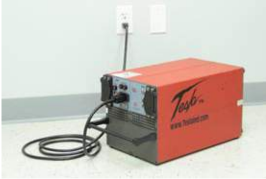
Figure 3.12.1 - Connecting TI1560 12-24 GPU to AC Power Supply
