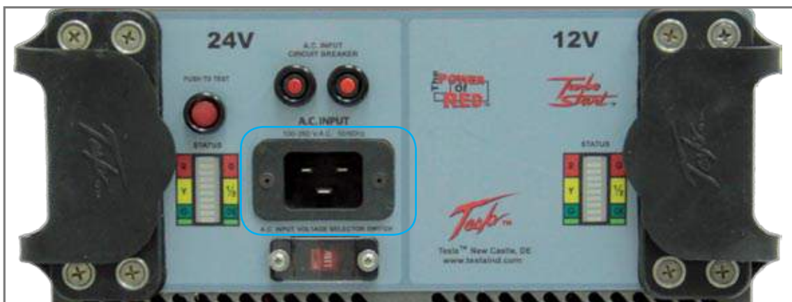
Figure 2.9.1 - AC Input Connector (outlined in blue)
