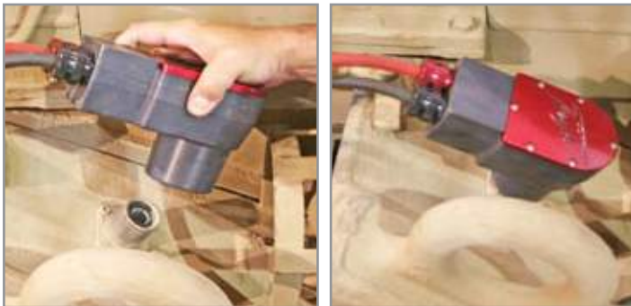
Figure 3.11.2 Attaching NATO DC Power Cable to vehicle
