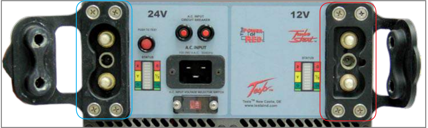
Figure 2.10.1 - 24 Vdc Output Connector (outlined in blue) /12 Vdc Output Connector (Outlined in red)
