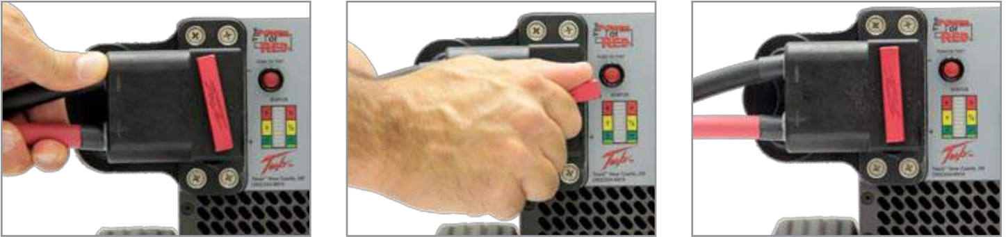
Figure 3.11.1 Attaching DC Power Cable to GPU
