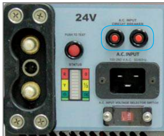
Figure 2.8.1 - AC Input Circuit Breaker (outlined in blue)
