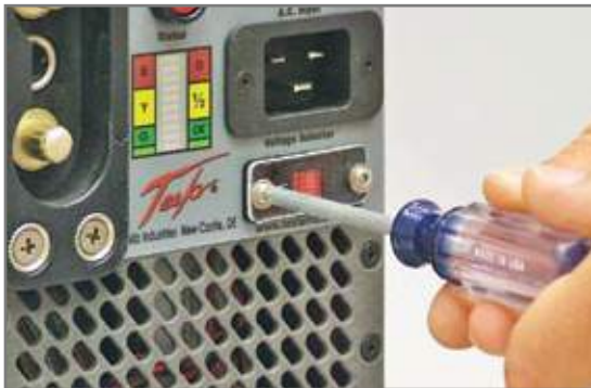
Figure 2.12.2 - Unscrew Protective Cover
