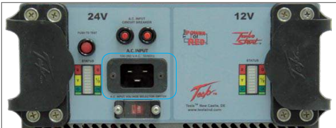
Figure 2.9.1 - AC Input Connector (outlined in blue)
