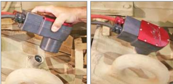
Figure 3.11.2 Attaching NATO DC Power Cable to vehicle
