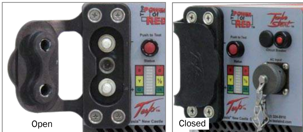
Figure 2.9.1 - 24 Vdc Output Connector Protective Cover
