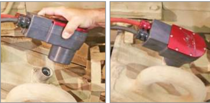
Figure 3.11.2 Attaching NATO DC Power Cable to vehicle
