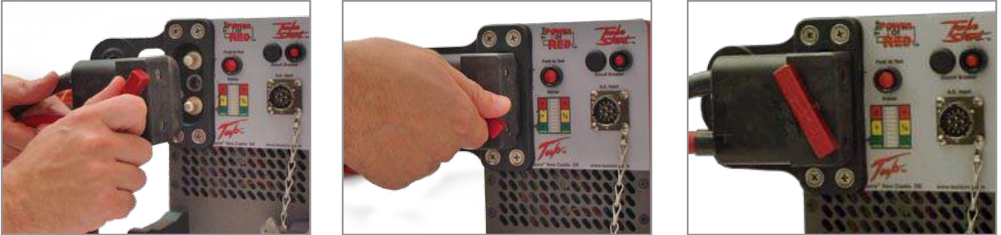
Figure 3.11.1 Attaching DC Power Cable to TI500 GPU-24
