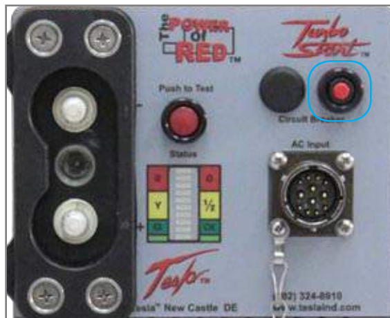
Figure 2.8.1 - AC Input Circuit Breaker (outlined in blue)
