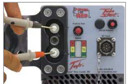
Figure 3.8.3 – Testing DC Receptacle
