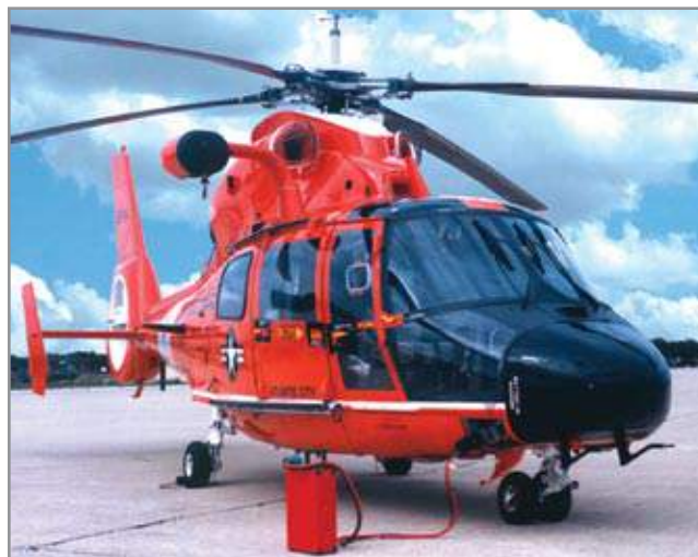
Figure 3.11.1 Starting aircraft with TI500 GPU-24
