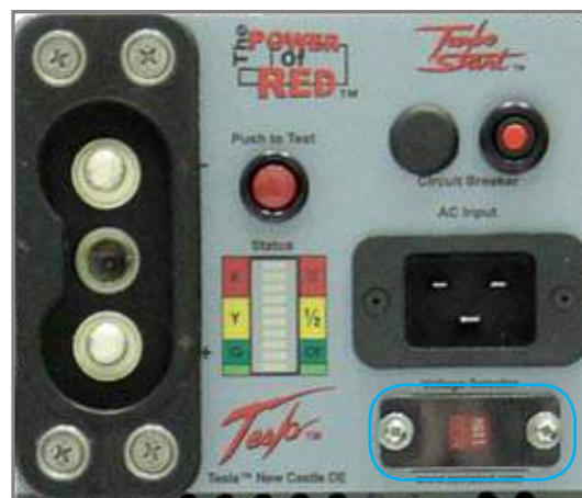
Figure 2.10.1 Input Voltage Selector Switch (outlined in blue)
