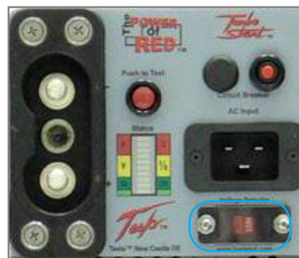
Figure 1.3.4 – TI2000 GPU-24 Input Voltage Selector Switch
