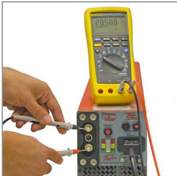
Figure 3.8.2 – Testing DC Receptacle
