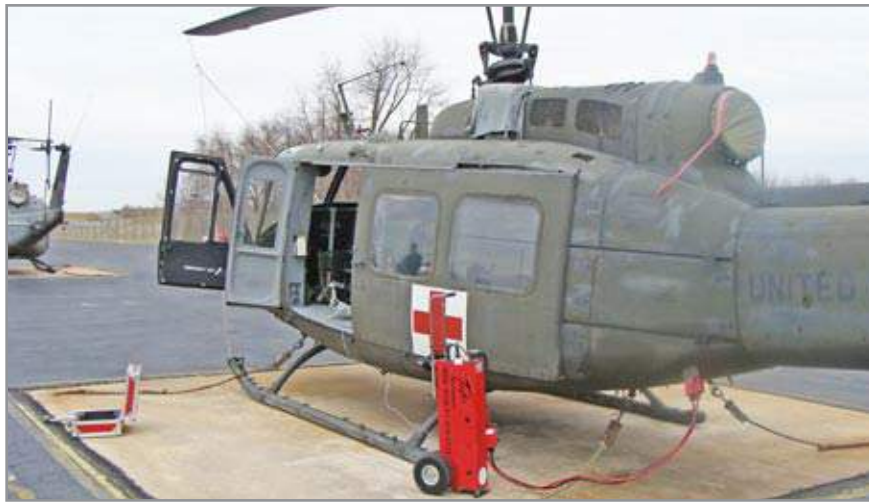
Figure 3.11.4 Starting UH-1 Huey Helicopter with TI2000 GPU-24
