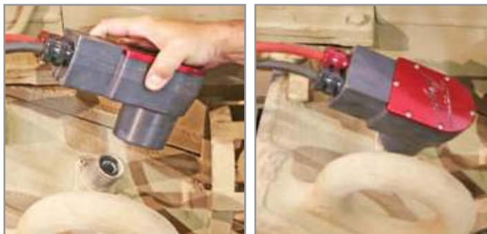
Figure 3.11.2 Attaching NATO DC Power Cable to vehicle
