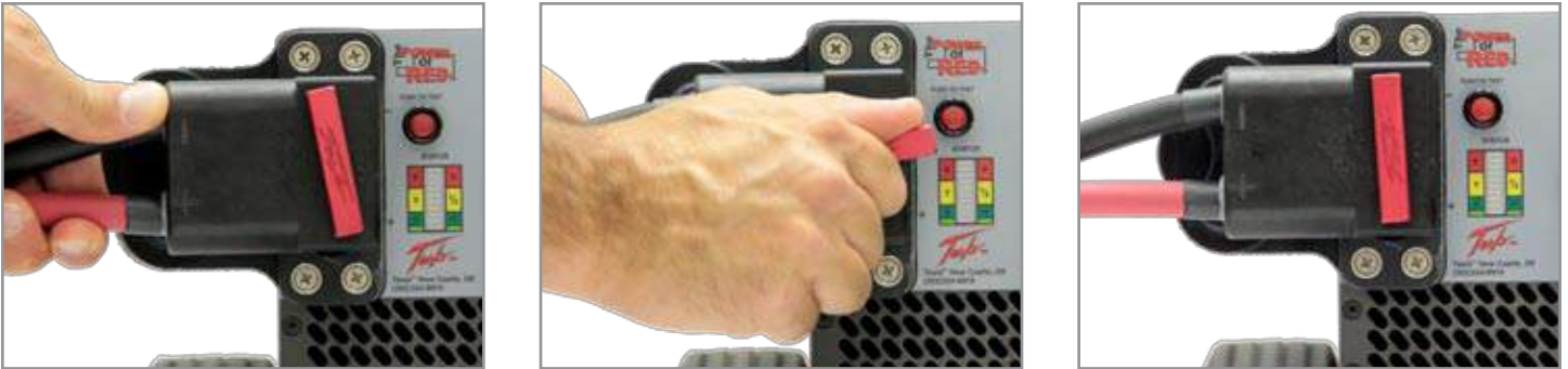
Figure 3.11.1 - Attaching DC Power Cable to TI2500 GPU-24
