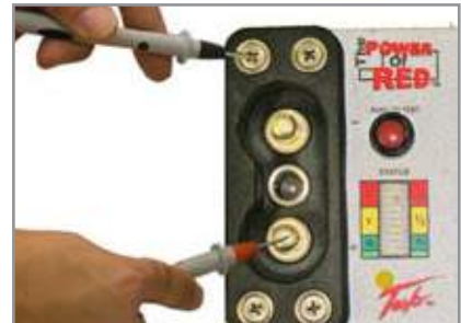
3. Place the negative probe to the fastener screw on the dc receptacle. Move the positive probe to the dc positive post. Multimeter should read 0 Volts.
