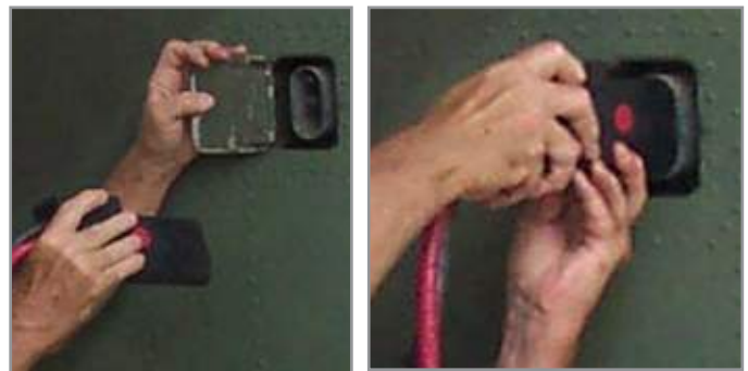
Figure 3.11.3 - Attaching DC Power Cable to aircraft
