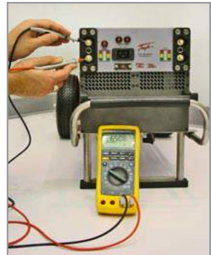
Figure 3.8.2 – Testing DC Receptacle
