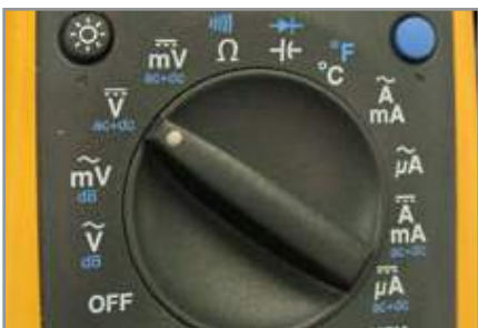
1. Set multimeter to Volts.
