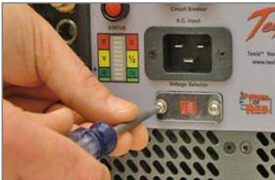
Figure 2.10.1 Unscrew Protective Cover
