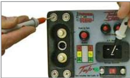
4. Move the positive probe to the fastener screw on the DC Receptacle. Multimeter should read less than 1Ω.
