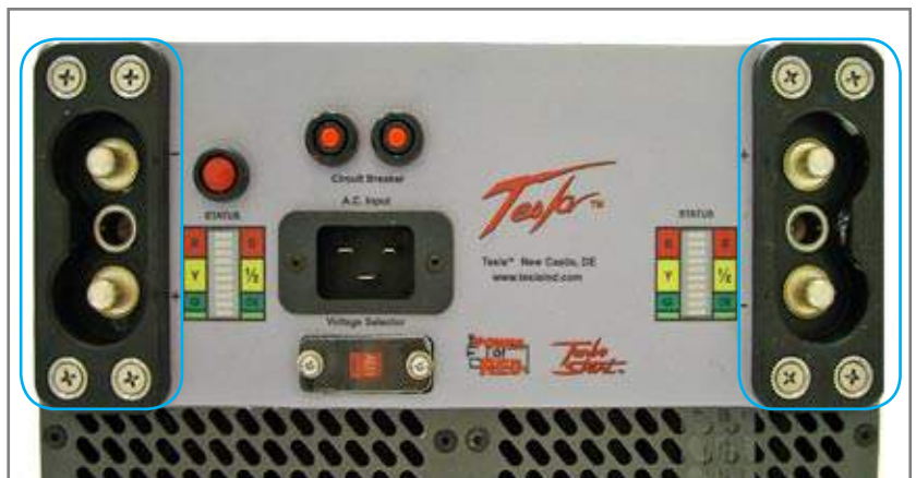
Figure 2.11.1 - 24 Vdc Output Connectors (outlined in blue)
