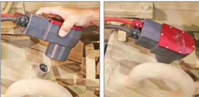
Figure 3.11.2 - Attaching DC Power Cable to vehicle
