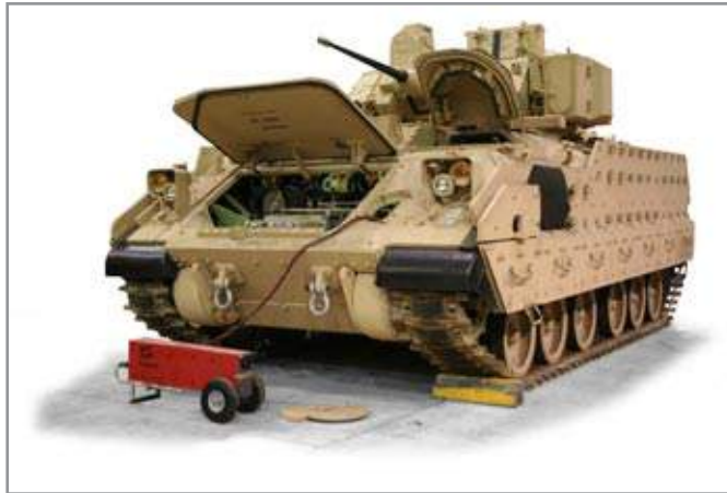
Figure 3.11.4 - Starting vehicle with TI2500 GPU-24
