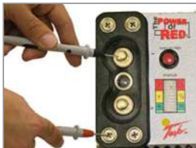
2. Place the positive probe to the fastener screw on the dc receptacle. Move the negative probe to the dc negative post. Multimeter should read 0 Volts.
