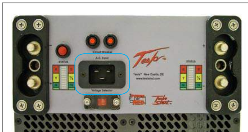
Figure 2.9.1 - AC Input Connector (outlined in blue)
