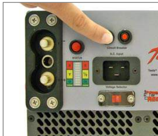
Figure 2.8.2 - Pressing Circuit Breaker
