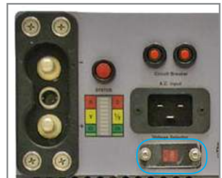
Figure 1.3.4 – TI2500 GPU-24 Input Voltage Selector Switch
