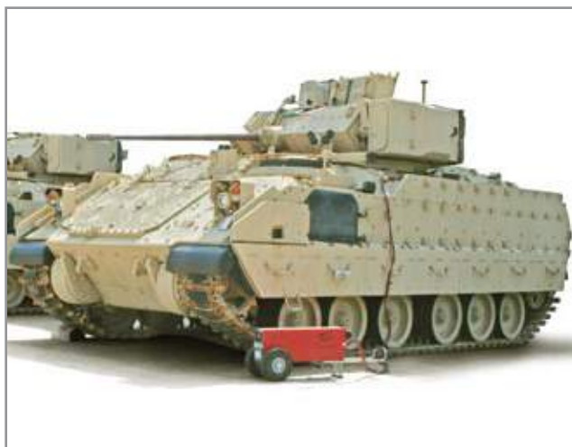
Figure 3.10.6 Starting Vehicle with TI3500 GPU-24
