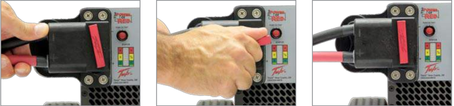
Figure 3.10.1 Attaching DC Power Cable to TI3500 GPU-24
