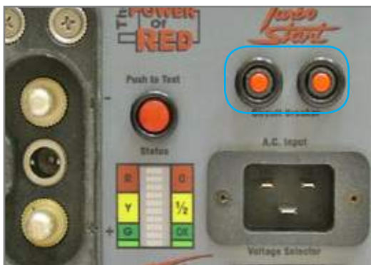
Figure 2.11.1 - AC Input Circuit Breakers (outlined in blue)
