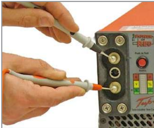
Figure 5.5.2 – Testing DC Receptacle
