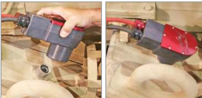
Figure 3.10.3 Attaching NATO DC Power Cable to vehicle
