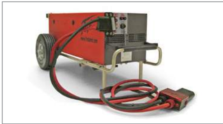
Figure 3.10.2 DC Power Cable Attached
