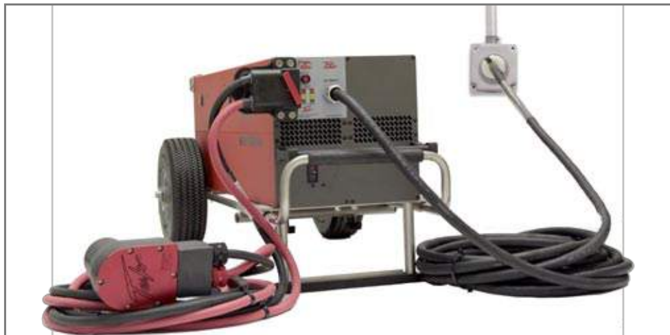
Figure 3.13.2 Connecting TI4100 GPU-24 to AC Power Supply with DC Power Cable Attached
