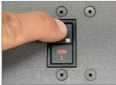
Figure 3.16.2 Switching Circuit Breaker OFF
