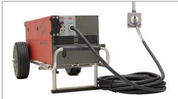
Figure 3.16.4 Plugging Into AC Single Phase Power
