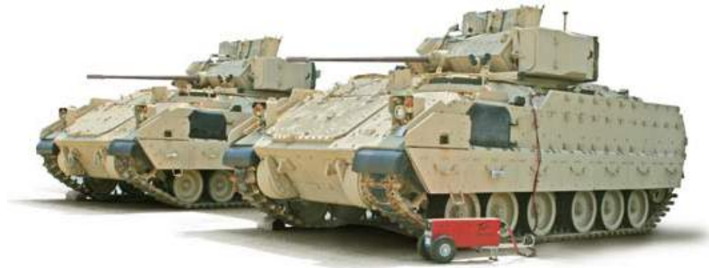
Figure 3.11.3 Starting vehicle with TI4100 GPU-24
