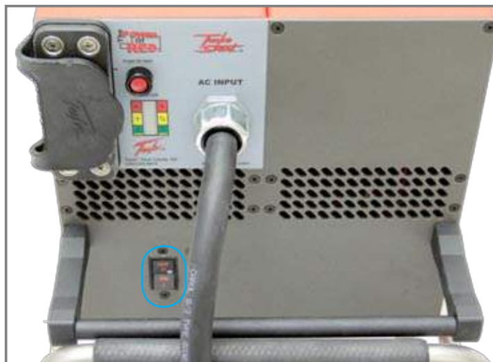
Figure 3.15.1 Circuit Breaker Selector Switch (outlined in blue)
