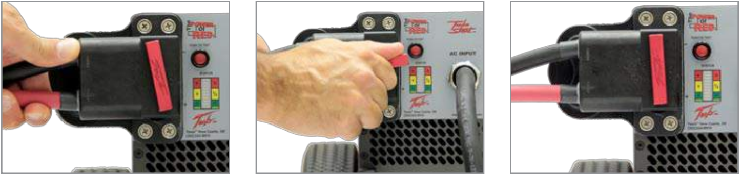
Figure 3.11.1 Attaching DC Power Cable to TI4100 GPU-24
