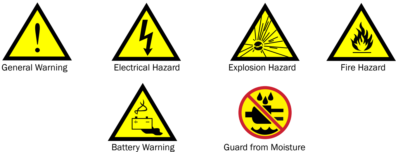
Figure 1.2.1 – Different types of hazard and caution symbols
