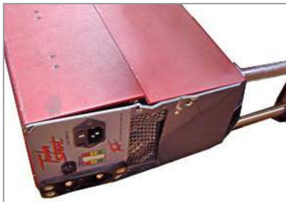
Figure 3.8.2 – Damaged Unit Misaligned Case with Bent Faceplate
