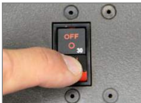
Figure 3.16.6 Switching Circuit Breaker ON
