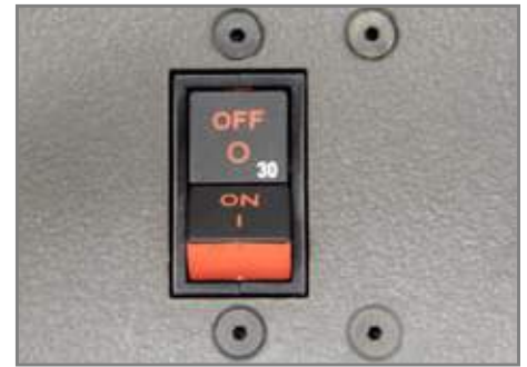
Figure 3.16.3 Circuit Breaker OFF
