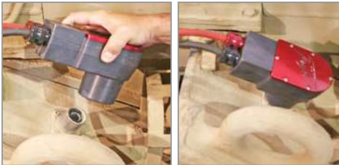
Figure 3.11.2 Attaching NATO DC Power Cable to vehicle
