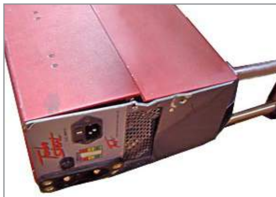
Figure 3.8.2 – Damaged Unit Misaligned Case with Bent Faceplate
