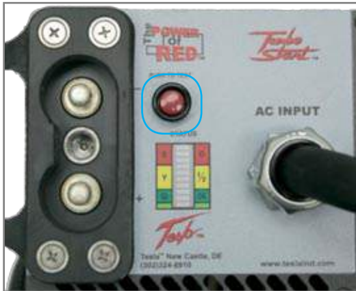
Figure 2.8.1 - “Push to Test” button location (outlined in blue)
