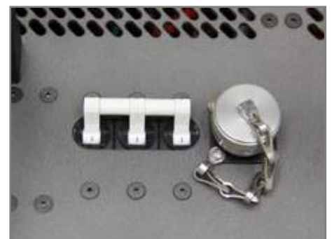
Figure 3.16.7 Circuit Breaker ON
