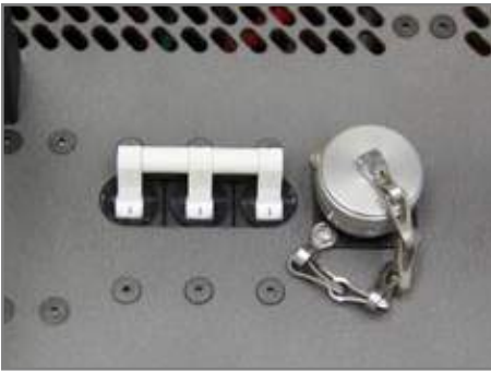
Figure 3.16.1 Circuit Breaker ON
