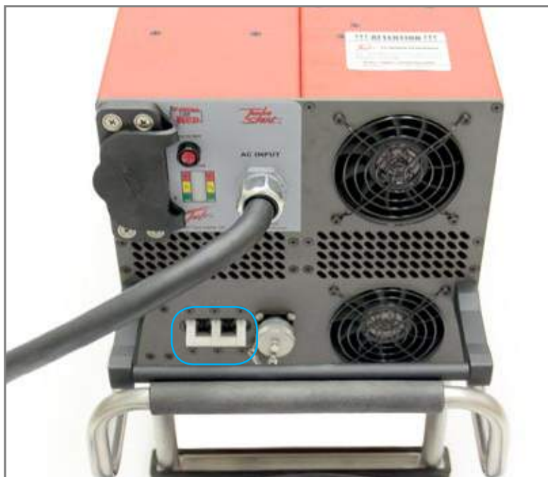
Figure 4.2.1 Circuit Breaker Selector Switch (outlined in blue)
