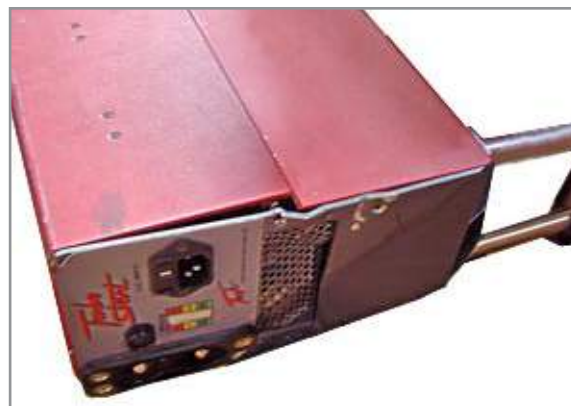
Figure 3.8.2 – Damaged Unit Misaligned Case with Bent Faceplate
