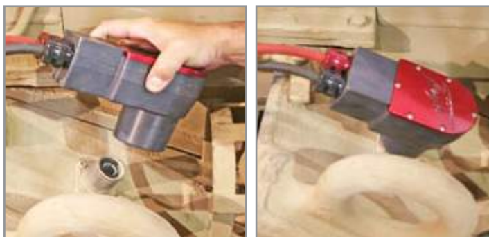
Figure 3.11.2 Attaching NATO DC Power Cable to vehicle
