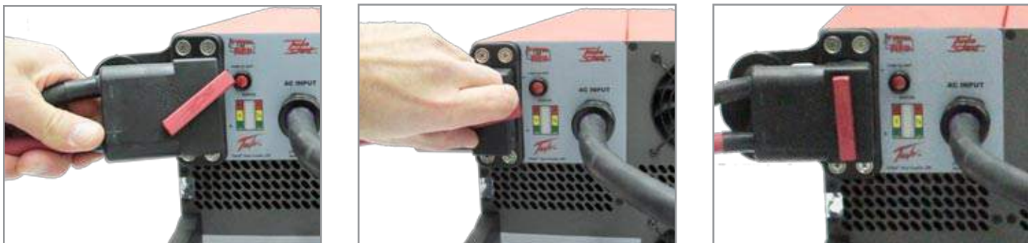
Figure 3.11.1 Attaching DC Power Cable to TI4200 GPU-24-PFC
