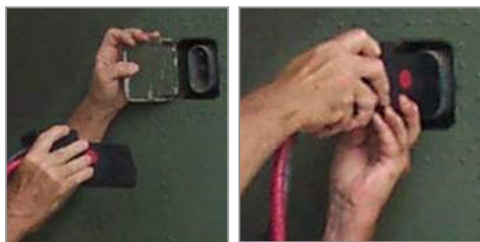
Figure 3.11.3 Attaching an Aviation DC Power Cable to aircraft
