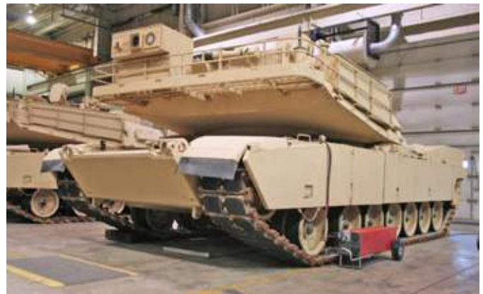
Figure 3.11.3 Starting vehicle with TI5200 GPU-24-PFC
