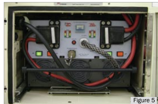
Figure 5 TI3950 GPU with DC Outputs
