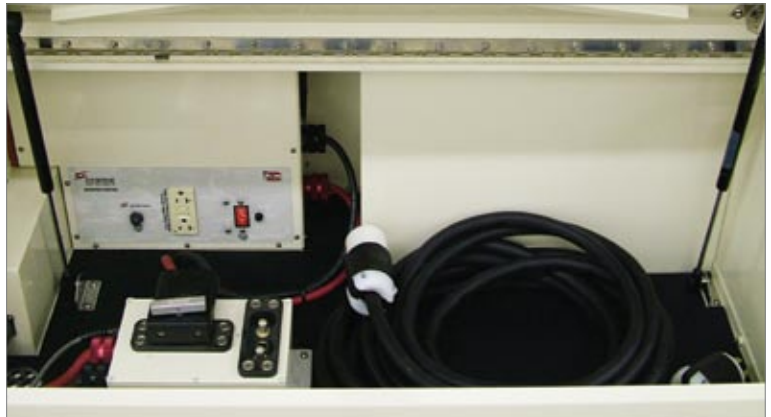
Figure 14: Storage Compartment, DC Output and Inverter Control Panel
