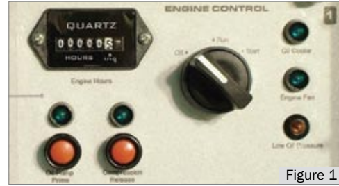
Figure 1 Engine Control Panel - Starter and Indicator LEDs
