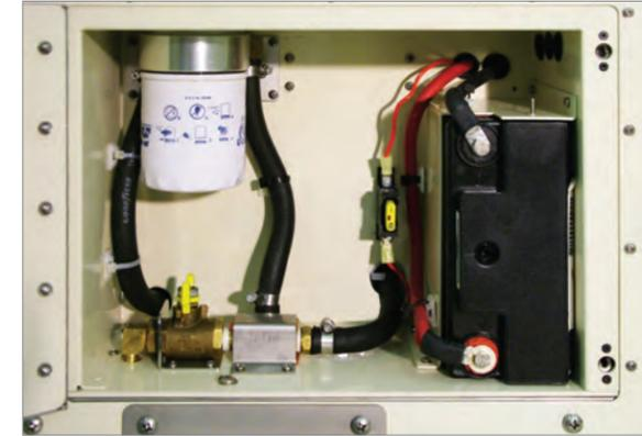
Figure 11: Oil Filter and Battery
