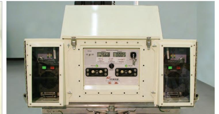
DC Receptacles and Dual Tesla™ TI3750 Ground Power Units
