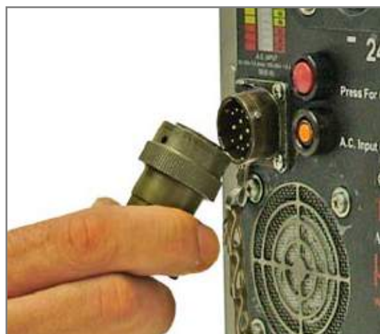
Figure 3.13.2 Attaching AC Line Cord
