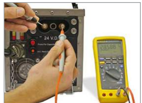
Figure 3.9.3 – Testing DC Receptacle
