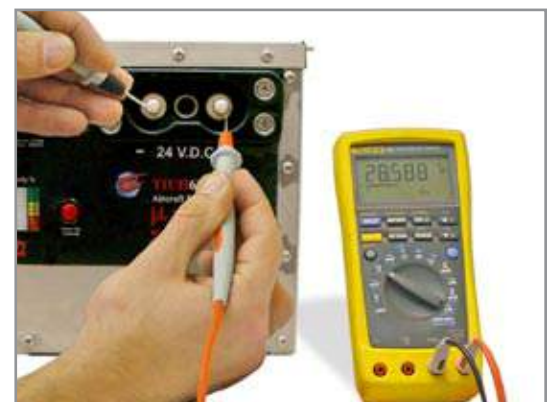
Figure 3.8.3 – Testing DC Receptacle
