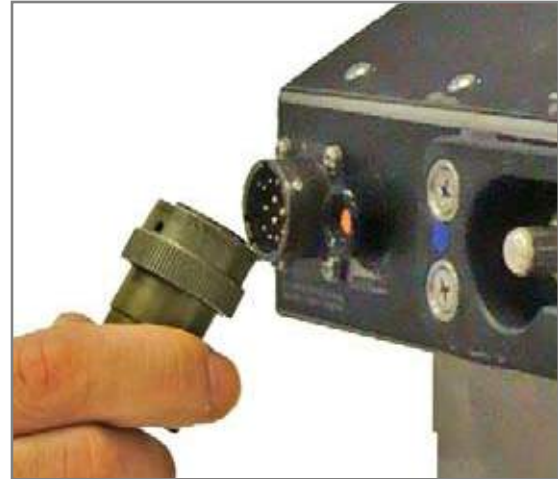
Figure 3.12.2 Attaching AC Line Cord
