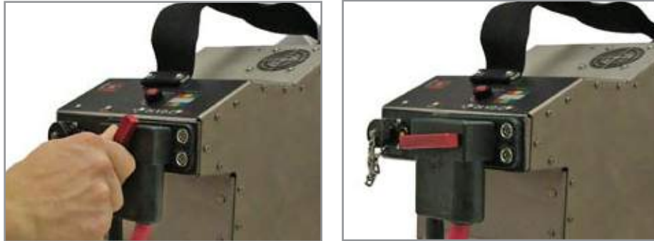
Figure 3.10.1 Attaching dc power cable to TI206 MPU-24
