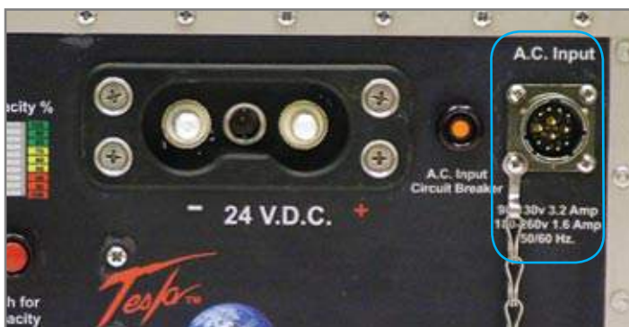
Figure 3.5.1 AC Input (outlined in blue)
