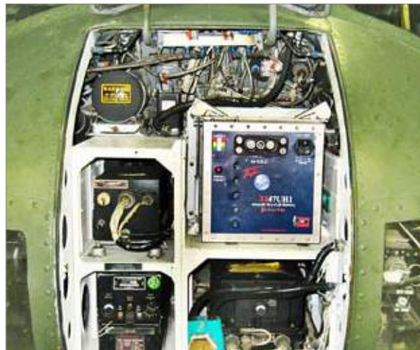
Figure 3.9.1 – TI47UH1 properly installed in a UH-1 Huey (DC Plug is not secured)
