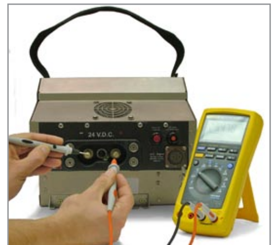
Figure 3.9.3 – Testing DC Receptacle
