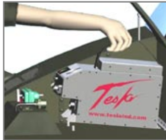
Figure 2.11.2 – Slide back flange into receiving lip
