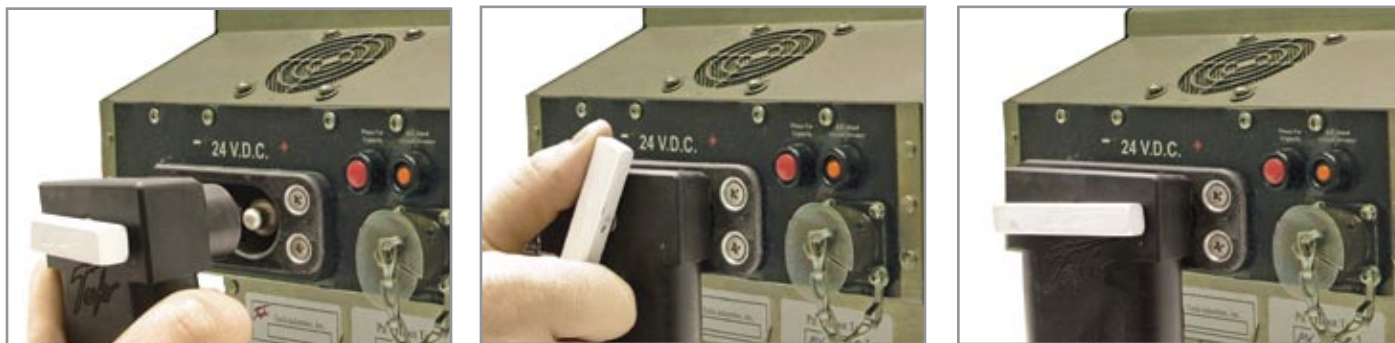
Figure 3.10.1 Attaching dc power cable to T147407 MPU-24
