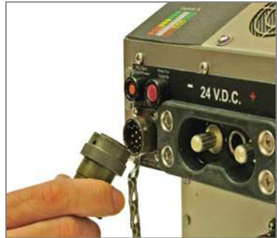
Figure 3.12.2 Attaching AC Line Cord
