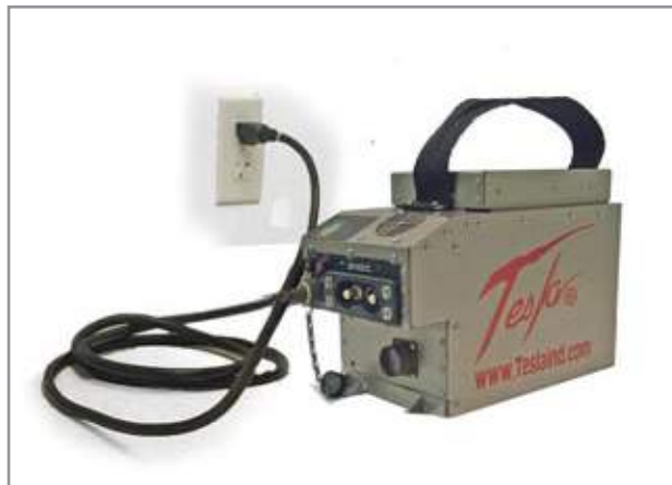
Figure 4.3.1 Connecting TI58D MPU-24 to ac power supply
