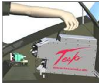
Figure 2.11.2 – Slide back flange into receiving lip
