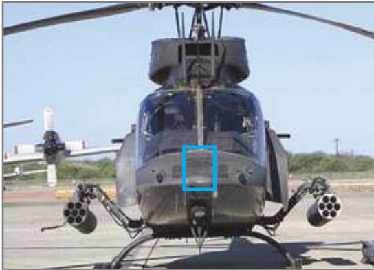
Figure 2.10.1 - OH58D Kiowa Warrior (Battery compartment highlighted in Blue)
