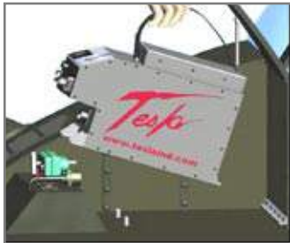
Figure 2.11.1 – Maneuver TI58D into battery compartment
