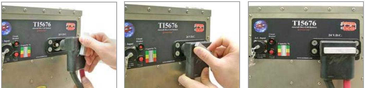
Figure 4.5.1 Attaching DC Power Cable to TI5676 MPU-24
