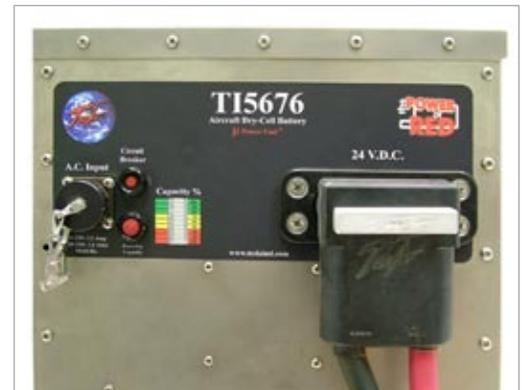
The battery charging system and ac-dc converter are built right into the TI5676 MPU.
