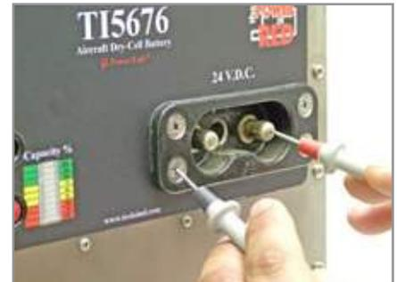
6. Move the positive probe to the dc positive post.
