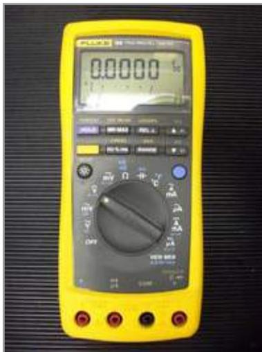
Figure 7.2.1 – Digital Multimeter
