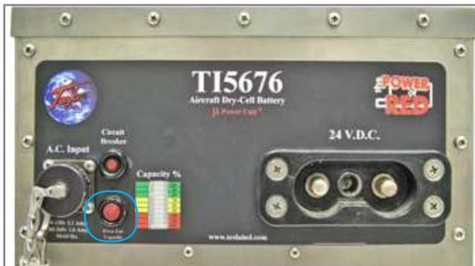
Figure 4.3.1 “Push to Test” button location
