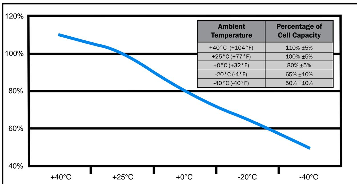
Figure 3.4.1 – Cell storage capacity versus ambient temperature
