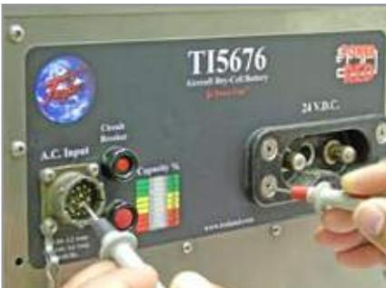
4. Move the positive probe to the fastener
