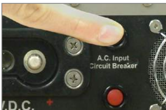
Figure 3.13.2 Pushing AC Input Circuit Breaker
