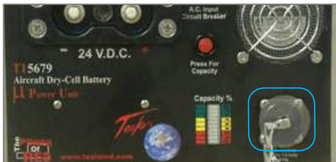
Figure 3.14.1 AC Input (outlined in blue)
