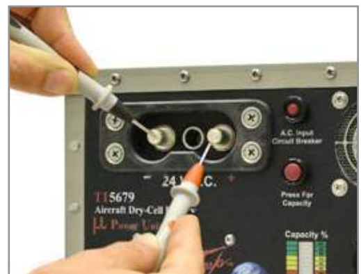
Figure 3.9.3 – Testing DC Receptacle
