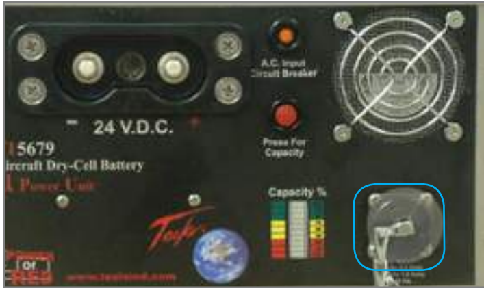
Figure 3.12.1 AC Input Connector (outlined in blue)
