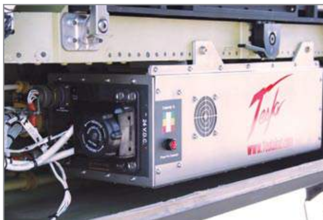
Figure 3.10.2 TIAH64D MPU-24 connected to dc power
