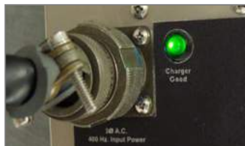
Figure 3.9.3 - “Charger Good” LED
