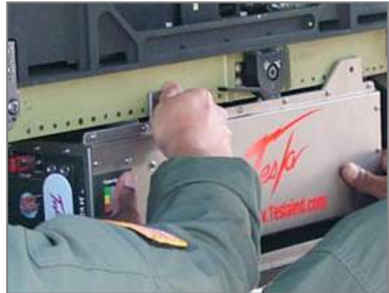
Figure 2.8.2 – Line up flanges over mounting holes and install screws and retained washers, and tighten
