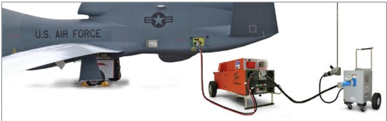
Figure 6.6.1 Connecting DC cable to aircraft and starting engine
