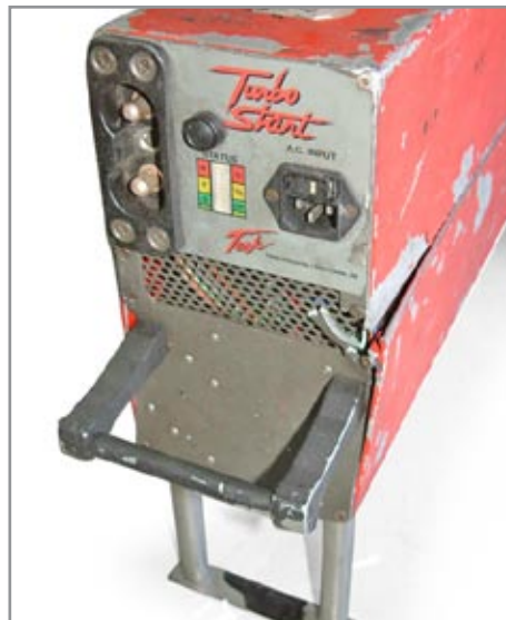
Figure 8.2.2 – Damaged Unit Misaligned Case with Bent Faceplate
