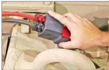
Figure 3.7.1 Attaching DC Power Cable to ground vehicle
