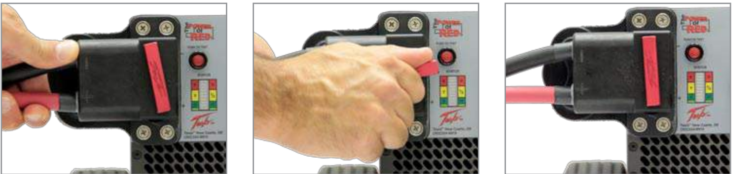
Figure 3.8.1 Attaching DC Power Cable to TI50A DC Power Supply
