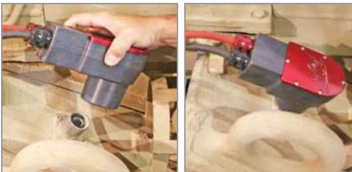
Figure 3.8.2 Attaching NATO DC Power Cable to vehicle
