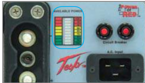
Figure 2.13.1 - “Available Power” LED Indicator location (outlined in blue)
