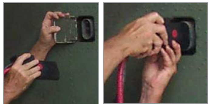
Figure 3.8.3 Attaching an Aviation DC Power Cable to aircraft
