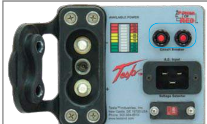
Figure 2.8.1 - AC Input Circuit Breaker (outlined in blue)
