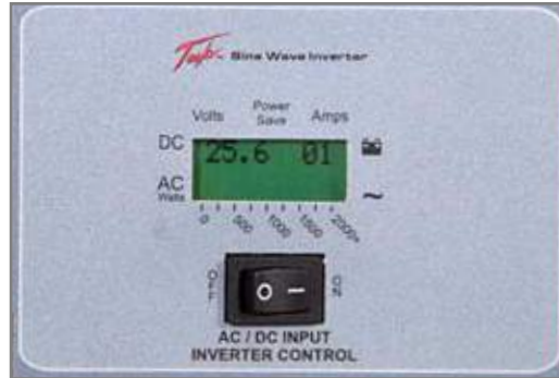
Figure 2.12.1 Inverter Display Panel
