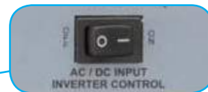
Figure 3.21.2 Inverter Display Panel with Switch set to “I” (ON) position.
