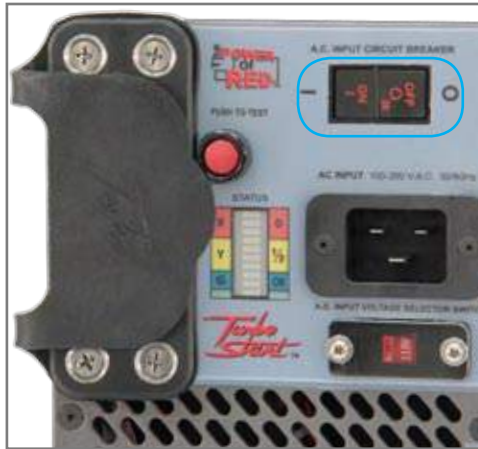
Figure 2.8.1 - AC Input Circuit Breaker (outlined in blue)
