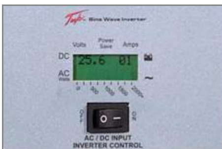
Figure 3.15.1 Inverter Display Panel with Switch set to “1” (ON) position.
