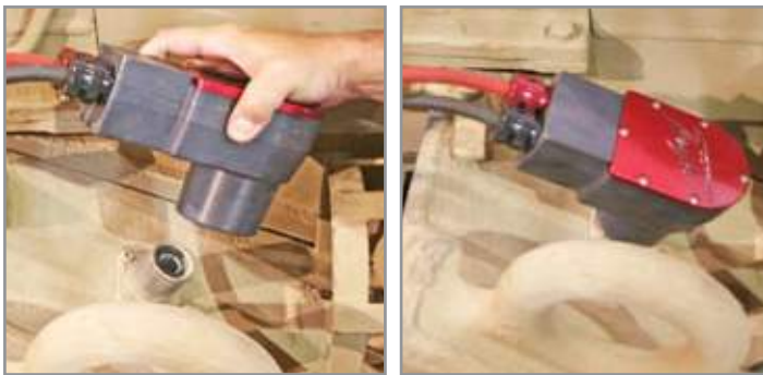
Figure 3.11.2 Attaching a NATO DC Power Cable to vehicle
