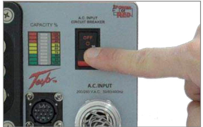
Figure 3.9.1 - Turning On AC Input Circuit Breaker
