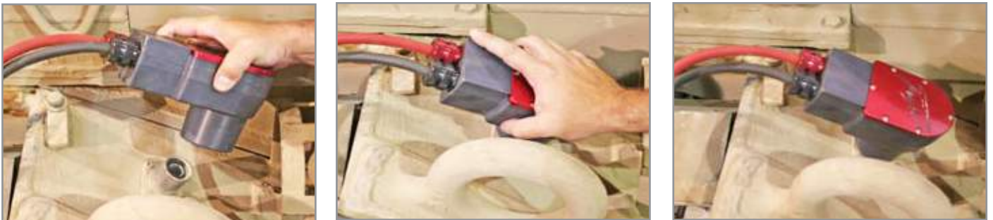
Figure 3.8.2 Attaching DC Power Cable to ground vehicle
