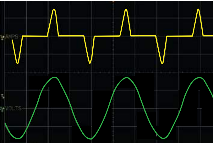
Figure 2.8.1 - Non-PFC Power Supply
