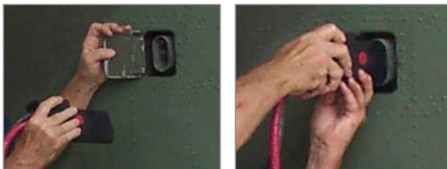
Figure 3.8.3 Attaching DC Power Cable to aircraft
