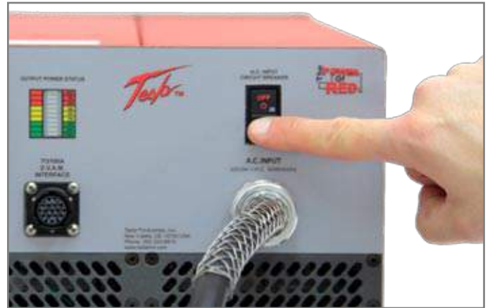
Figure 3.9.1 - Turning On AC Input Circuit Breaker
