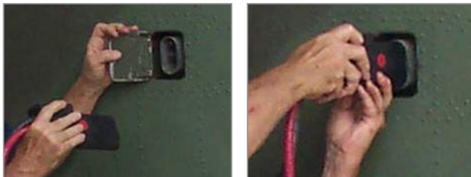
Figure 3.7.3 Attaching DC Power Cable to aircraft
