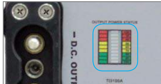
Figure 2.13.1 - Output Power Status Indicator location (outlined in blue)
