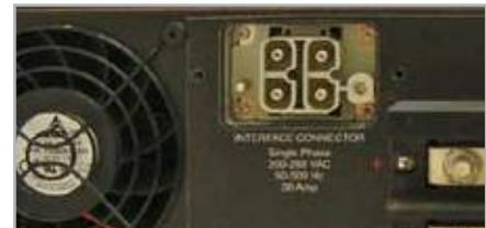
Figure 2: AC Input and Cooling Fan
