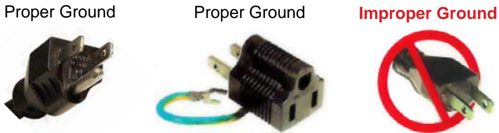
Figure 4.2.1- Illustrations of proper and improper grounding
