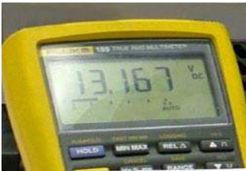
Figure 6.2.4 – Multimeter reading typical 12 V power cell voltage
