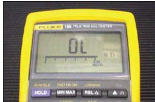
Figure 6.2.3 – Multimeter reading open circuit
