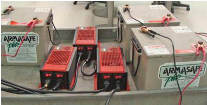
Battery Charger/Conditioner shown charging 12 V Hawker batteries using the Quick Disconnect Cable with Alligator Clips.
