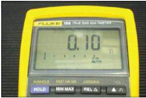
Figure 6.2.2 – Multimeter reading continuity
