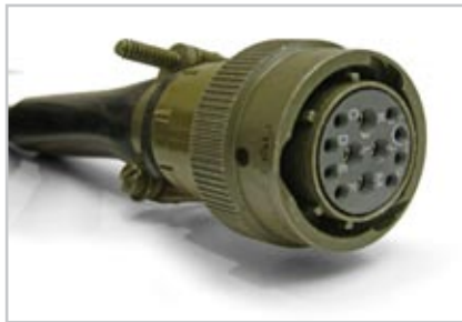
Figure 2.3.1 – Universal AC Input Cannon Plug
