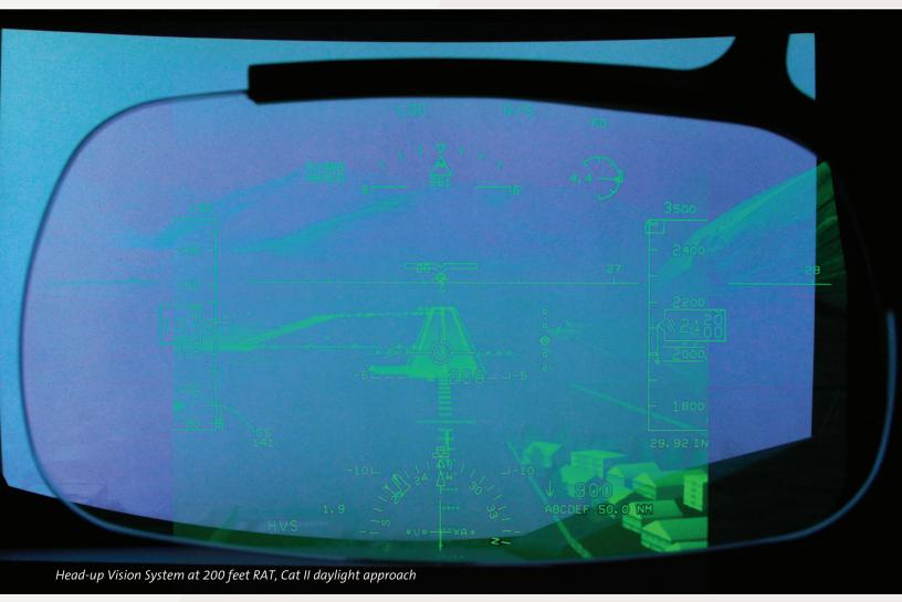
Innsbruck, Austria, CAT II daylight approach: Rockwell Collins' Head-up Vision System (HVS) is the industry's first integration of our Head-up Guidance System (HGS™) with our Synthetic Vision System (SVS) and our Enhanced Vision System (EVS) wideband, multispectral camera. The combination of SVS fused with multispectral EVS on a "head-up, eyes-out" display that conforms to the outside world provides a powerful safety tool.
