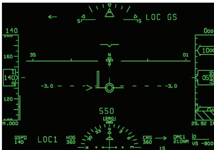
Figure 1: The HUD displays both conventional flight information and HUD-specific conformal symbols
