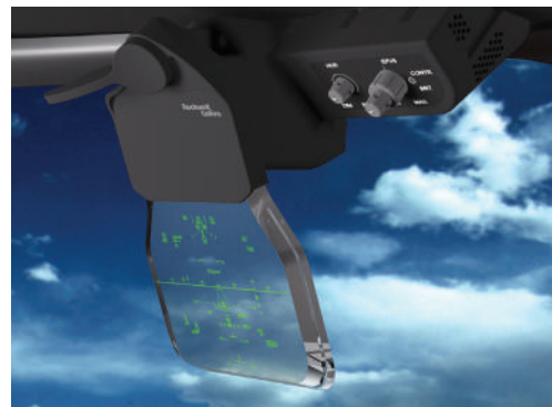
Figure 6: The HGS-3500 Display Unit is installed above the windscreen.
