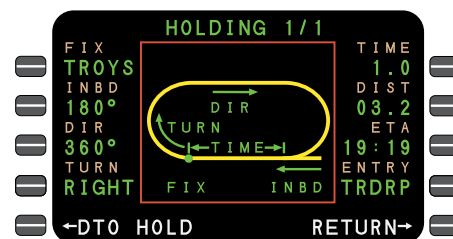
Holding patterns are accurately flown through the SBAS-FMS automatically, complete with appropriate entry procedure: direct, parallel or teardrop.
