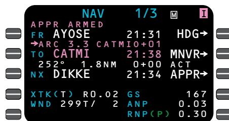
The RNP associated with the current leg is displayed on the NAV pages. The RNP value is obtained from the navigation database when provided for that leg; otherwise it is the FMS default value for the current phase of flight.
