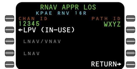
SBAS-FMS Approach Mode provides ILS-like guidance with LPV, LNAV/VNAV and LNAV level of service for RNAV (GPS) approaches.
