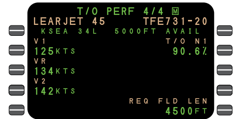
T/O speeds, runway length and N1 settings from AFM Performance Charts stored in memory.
