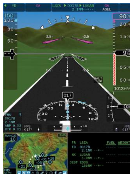
PFD with Arc HSI, Left Inset with SVS and Traffic, Right Inset with Flight Plan Data
