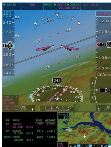
PFD with Arc HSI, Left Inset with Flight Plan Data, Right Inset with SVS
