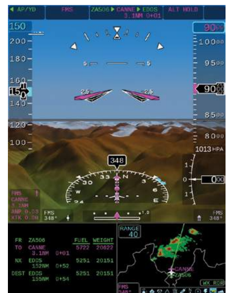
PFD with Arc HSI, Left Inset with Flight Plan Data, Right Inset with Map and Weather
