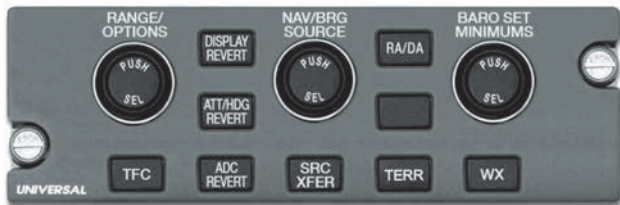
PFD Combined Display Control Panel
