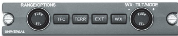
Display and Radar Control Panel
