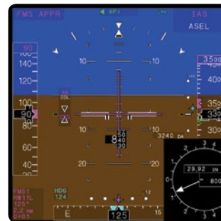
Full Primary Flight Display with Cross Pointer Overlay and Low Altitude Mode
