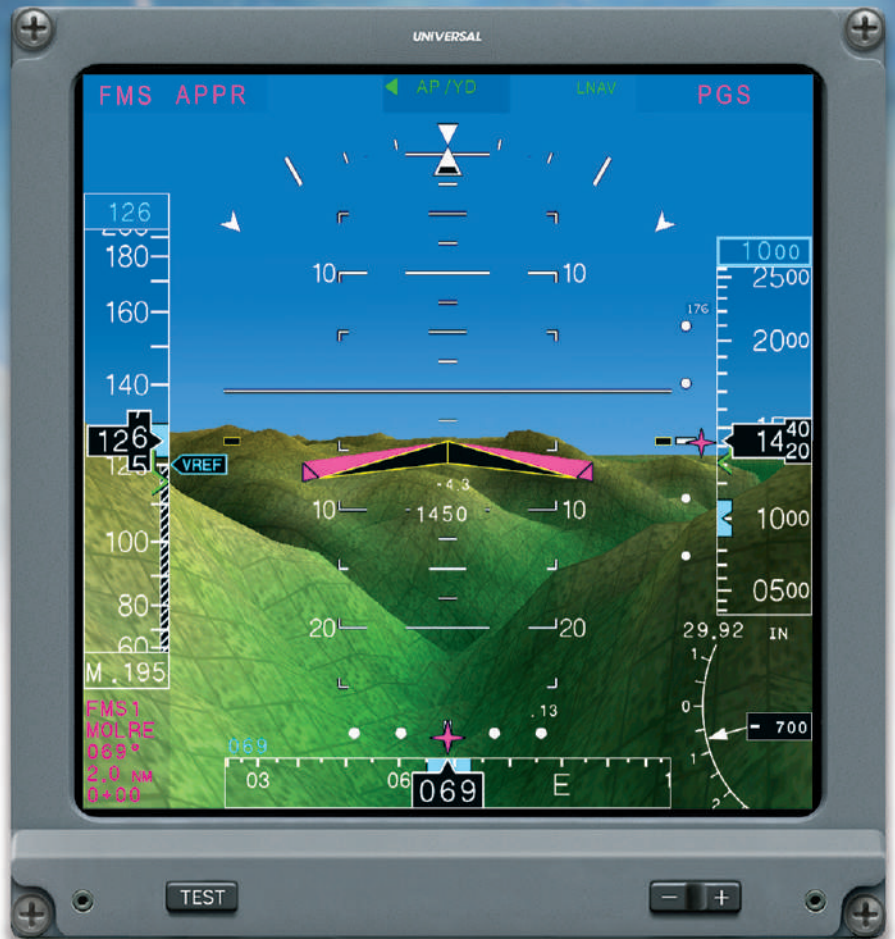
SVS Egocentric View shown on EFI-890R Primary Flight Display
