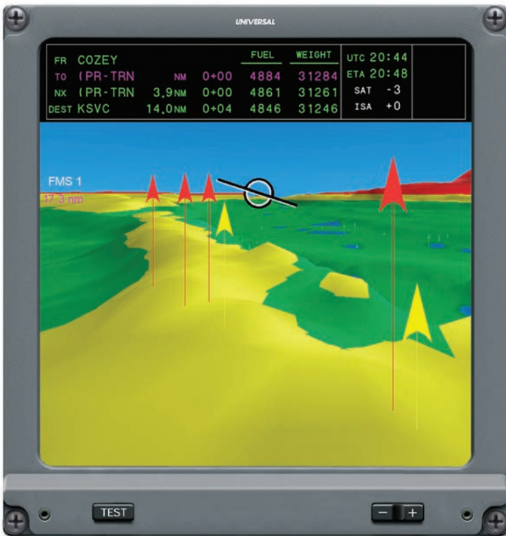
A unique 3-D Perspective View depicts terrain and obstacles as it would appear if viewed from 1,000 meters (3,281 feet) behind the aircraft. The circle at the top of the waypoint depicts the altitude constraint. A perspective correct 200-foot high triangle with a concave base and a pole that connects the triangle and the ground represents the 3-D Perspective View Obstacle symbol.
