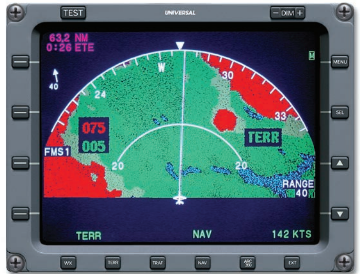
A map view of terrain can be output using ARINC 708 or WXPD formats for interface with various existing radar displays as well as existing EFIS. The maximum terrain elevation is also displayed.
